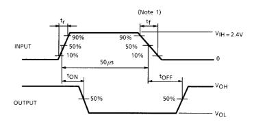
Note 1: Pulse Width 50  $\mu$ s, Duty Cycle 10% Output Impedance 50  $\Omega$ ,  $t_f \le$  5ns,  $t_f \le$  10 ns
