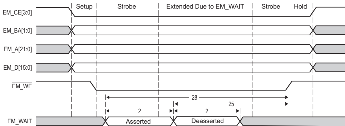
Figure 9-59 EMIF16 EM_WAIT Write Timing Diagram
