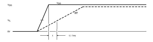
Adjust condenser value which is set  $\overline{\text{INT}}$  pin to the period while  $\overline{\text{INT}}$  pin is "L" level is longer than 1ms when power on.
