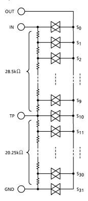
• Volume step and attenuation (Attenuation is as follows when resistor (3.9k $\Omega$ ) is connected between TP pin and GND pin.)
