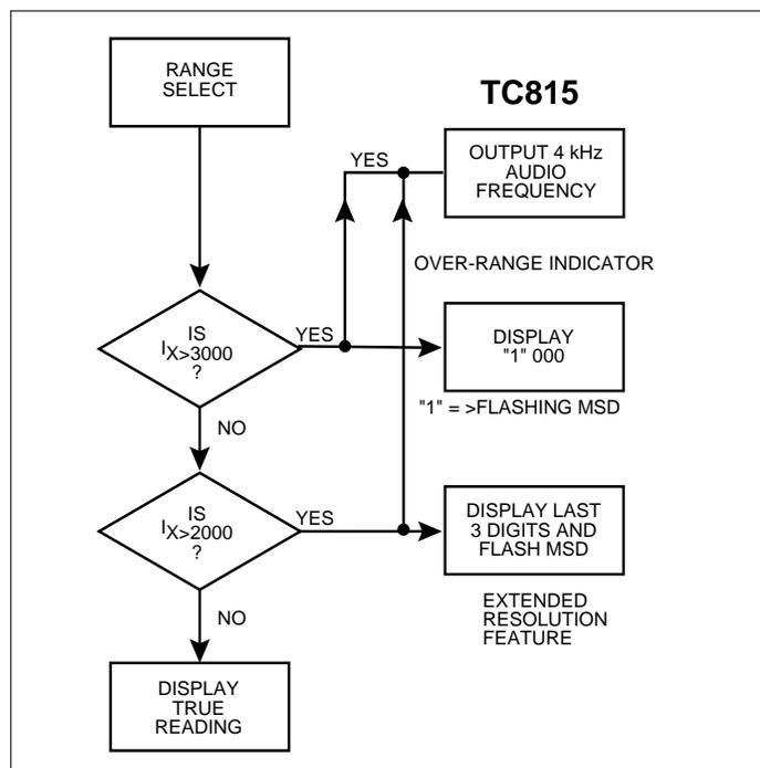
Figure 7. Manual Range Selection; Current Measurements
