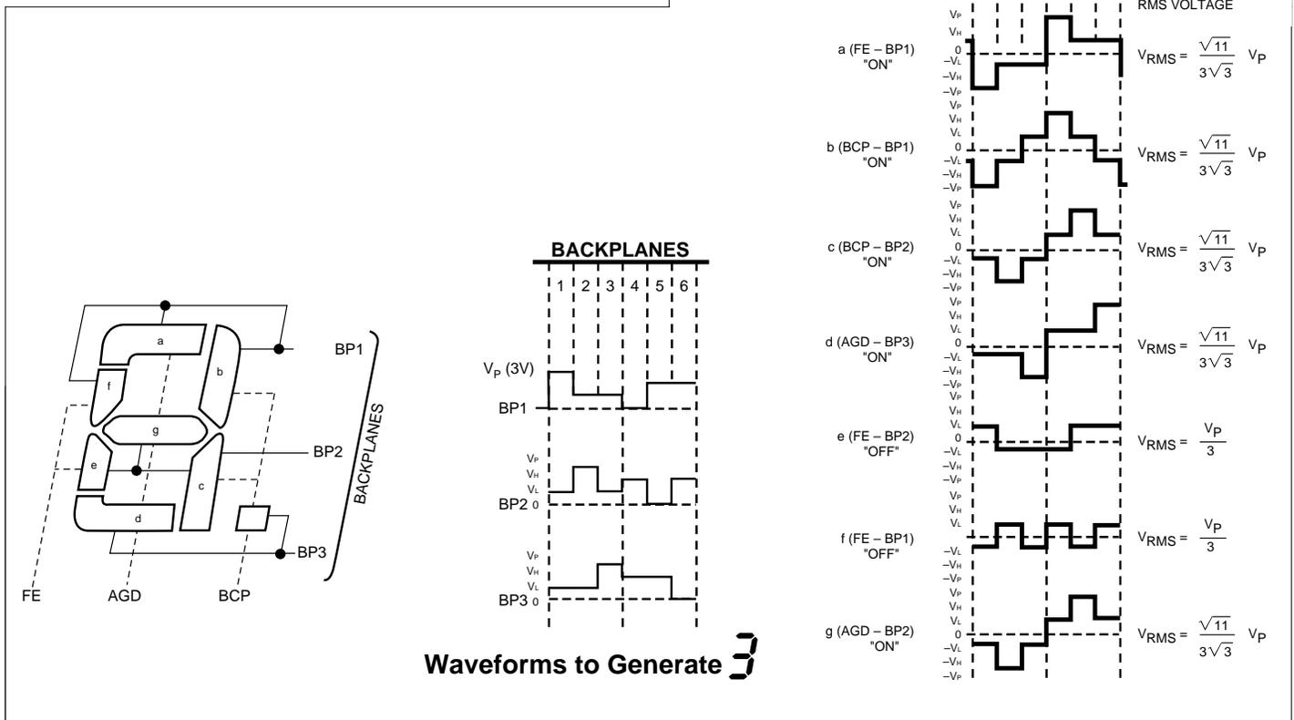
Figure 13. Triplex LCD Drive Waveforms
