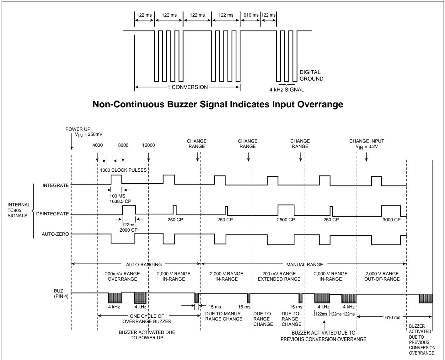
Figure 15. TC815 Timing Waveform for Buzzer Output
