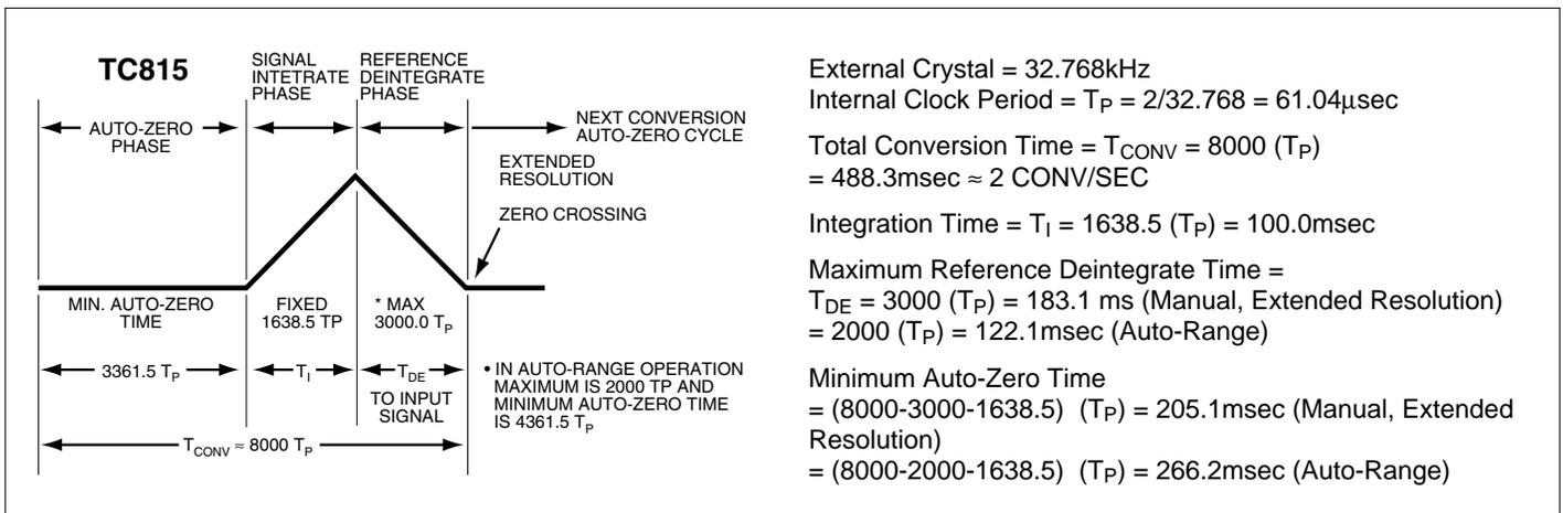
Figure 5. Basic TC815 Conversion Timing
