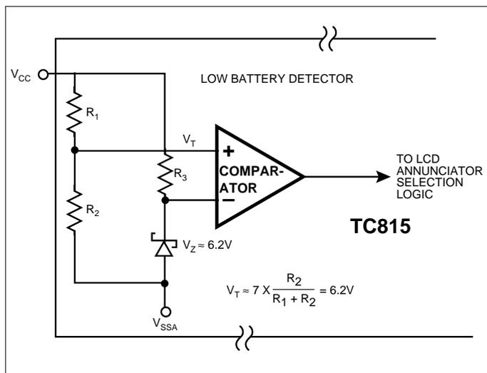
Figure 11. Low Battery Detector
