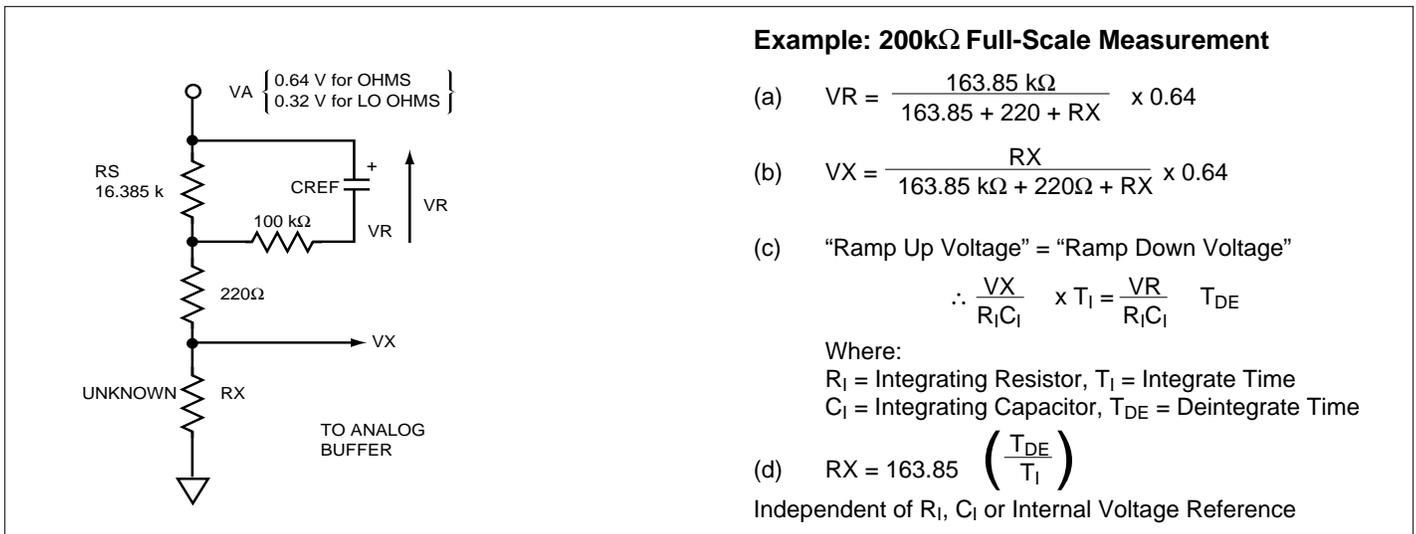
Figure 4. Resistance Measurement Accuracy Set by External Standard Resistor
