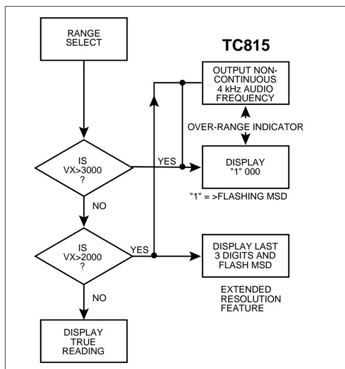
Figure 8. Manual Range Selection; Voltage Measurements
