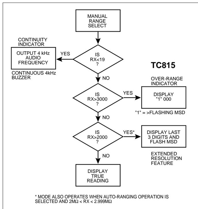
Figure 6. Manual Range Selection; Resistance Measurements
