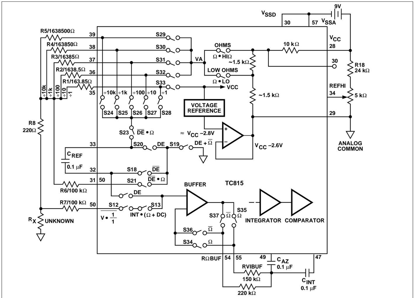
Figure 3: Ratiometric Resistance Measurement Functional Diagram
