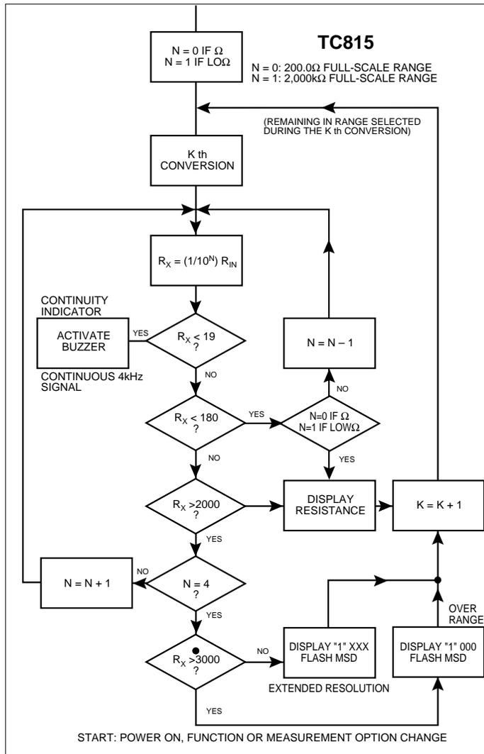
Figure 10. Auto-Range Operation; Resistance Measurement
