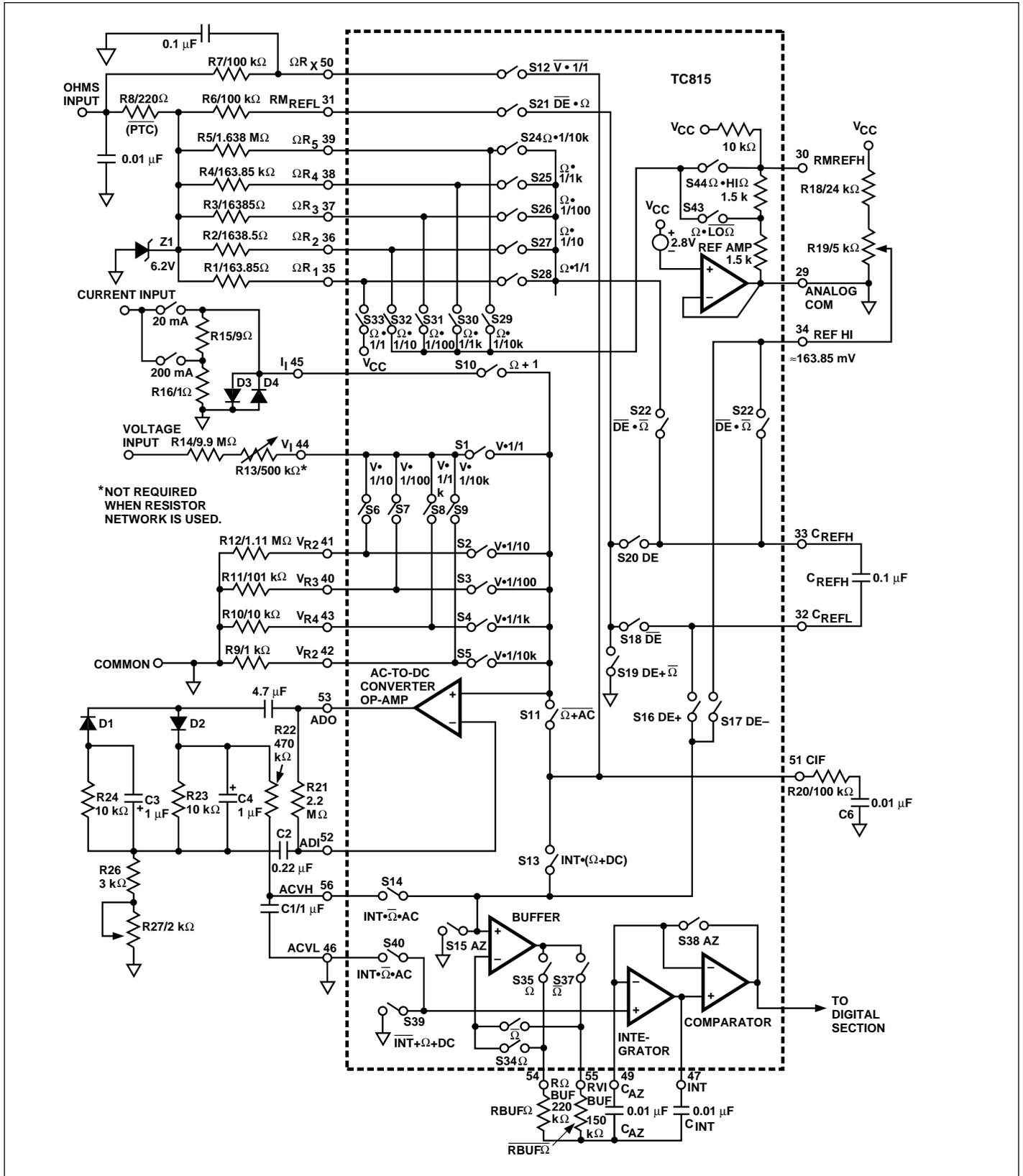
Figure 2: TC815 Analog Section
