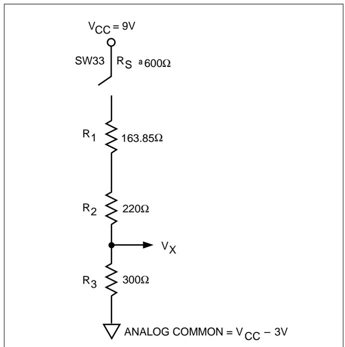
Figure 16. RΩBUF Calculation (200 Ω Manual Operation)
