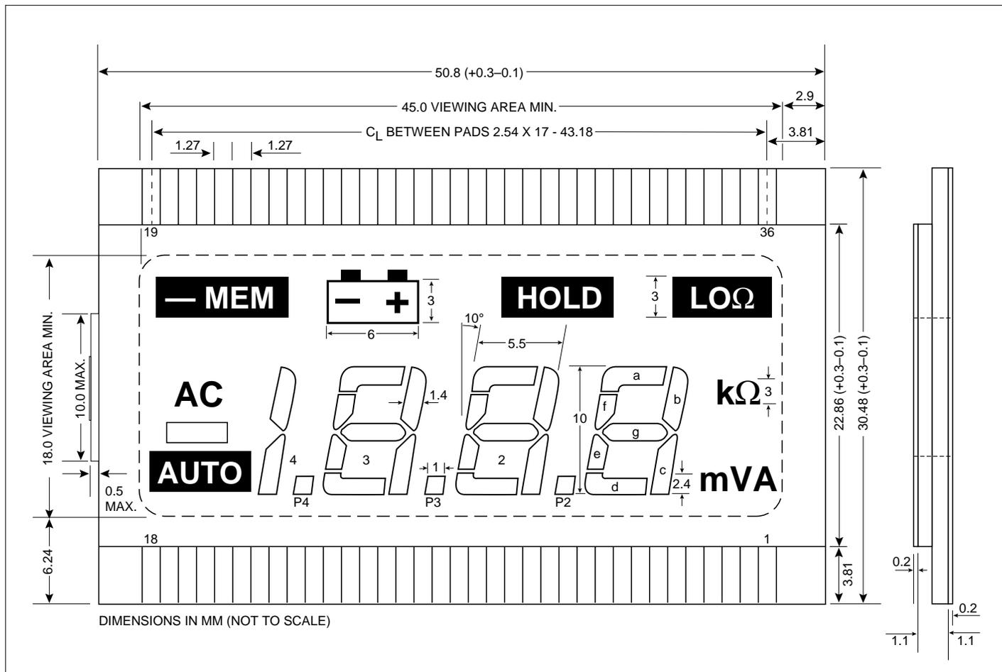
Figure 14. Typical LCD Display Configuration TC815 Triplex
