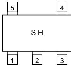
**Pin Connection (top view)**
