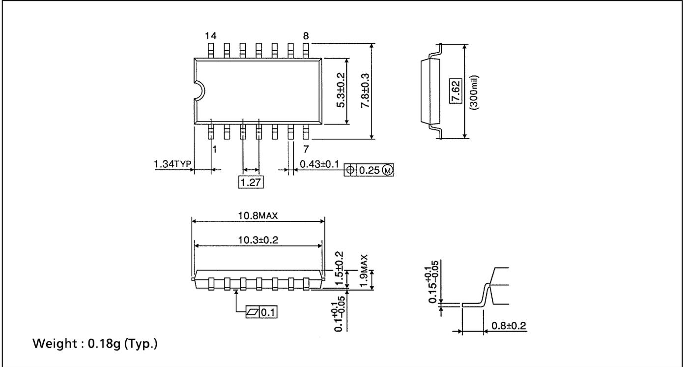
**SOP 14PIN (150mil BODY) PACKAGE DIMENSIONS (SOP14-P-150-1.27)**
