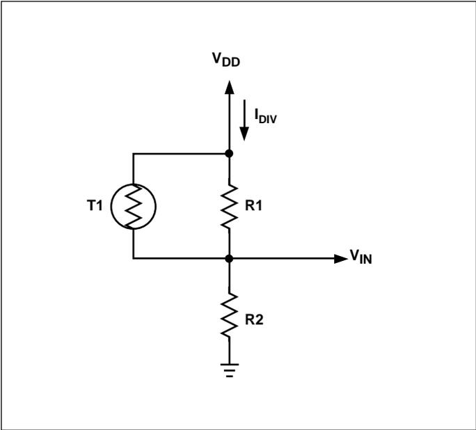
Figure 3. Temperature Sensing Circuit
