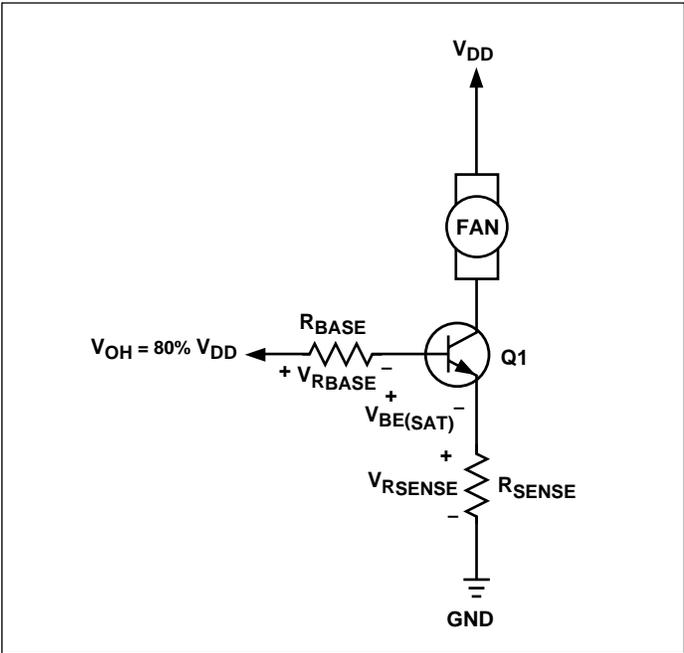
Figure 5. Circuit for Determining RBASE
