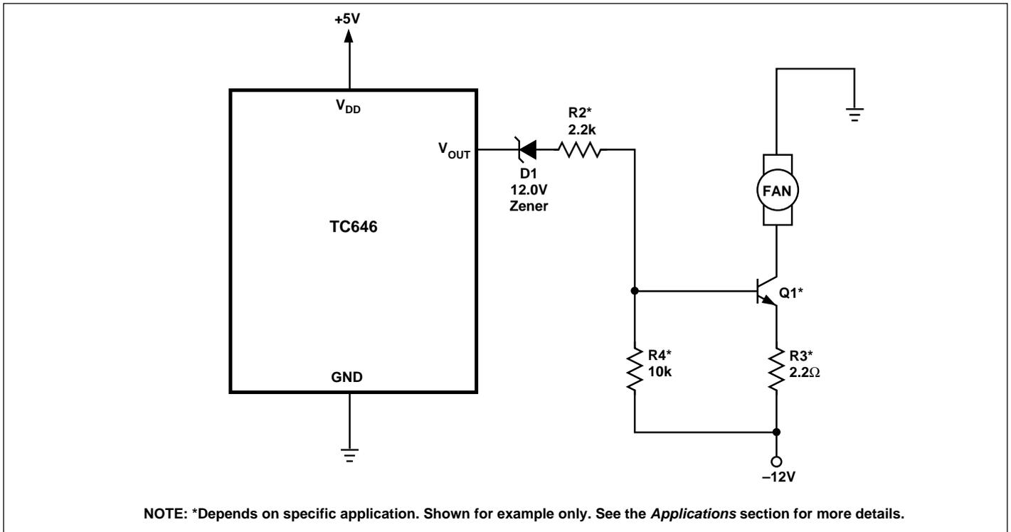
Figure 9. Powering the Fan from a Negative Supply
