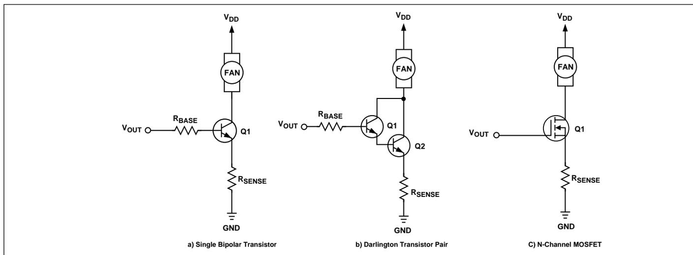
Figure 8. Output Drive Transistor Circuit Topologies
