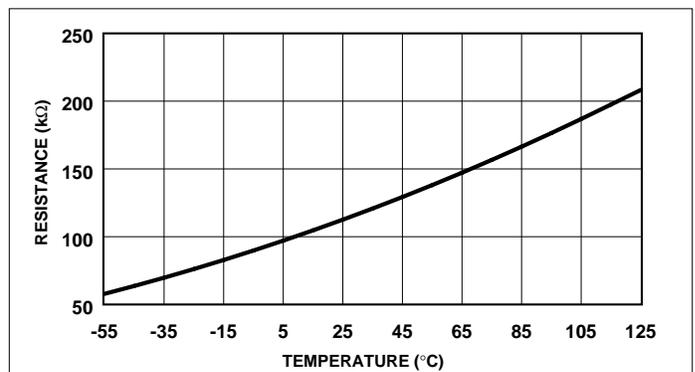
Figure 1. Programming Resistor Values vs. Temperature
