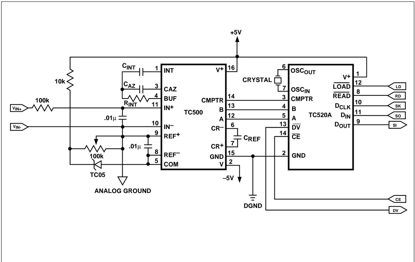
Figure 3. Typical System Application
