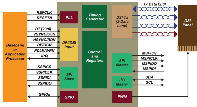
The TC358763XBG supports data transfer from input port (Host interface) to output port (Display Interface) as shown in the following use case scenarios:
