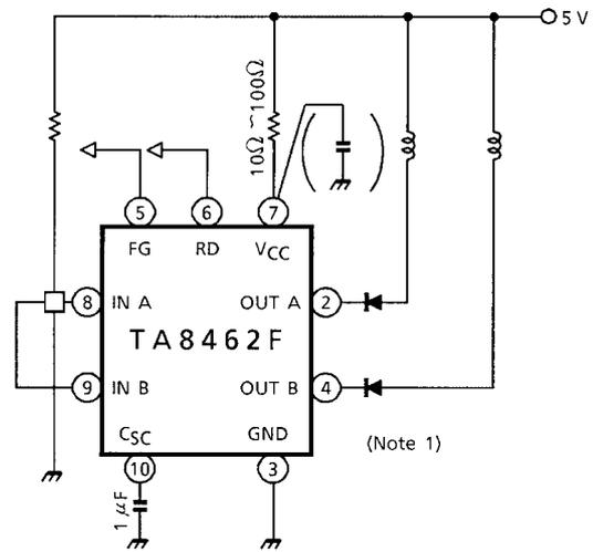
Note 1: In order to prevent the mutual induction of a motor, connect a additional diode between each output to motor.
