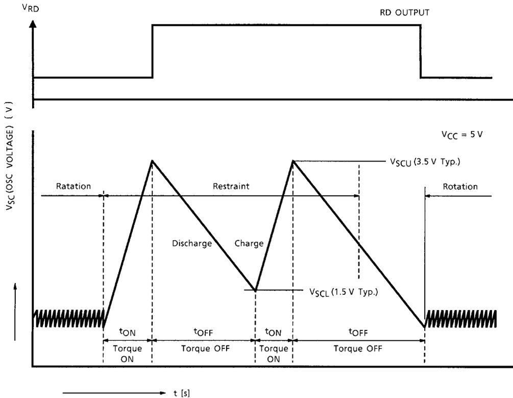
**Fig.1 Auto mAtic Self Rotation Recovery Circuit Operation**
