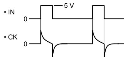
The capacitor coupling allows reset pulses to be supplied intermittently from the  $\overline{\text{RESET}}$  pin whether the input level (IN) is high or low.
