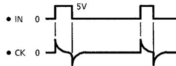
The capacitor coupling allows reset pulses to be supplied intermittently from the  $\overline{RESET}$  pin whether the input level (IN) is high or low.
