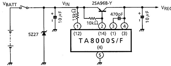
**EXAMPLE OF APPLICATION CIRCUIT USING DARLINGTON TRANSISTOR**
