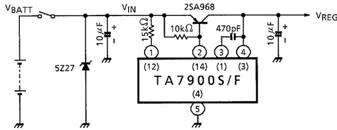
**Example of Application Circuit Using Darlington Transistor**
