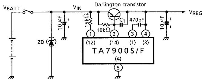
\*: Select a  $C_1$  value according to the working condition -- typically above 2000pF. Insert ZD when necessary.
