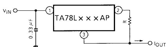
$$I_{OUT} = \frac{V_{OUT}}{R} + I_B$$
