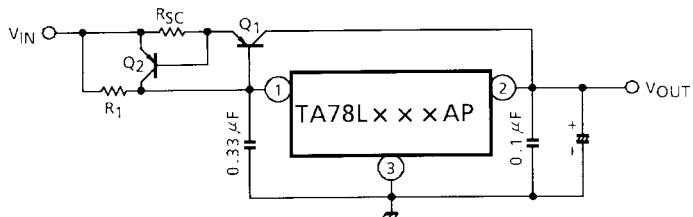
$$R_{SC} = \frac{V_{BE2}}{I_{SC}}$$
