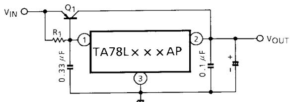
Use a required radiation plate for Q<sub>1</sub>.
