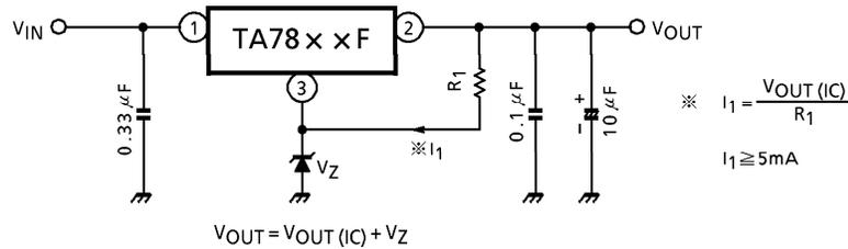
(b) Voltage boost by use of resistor
