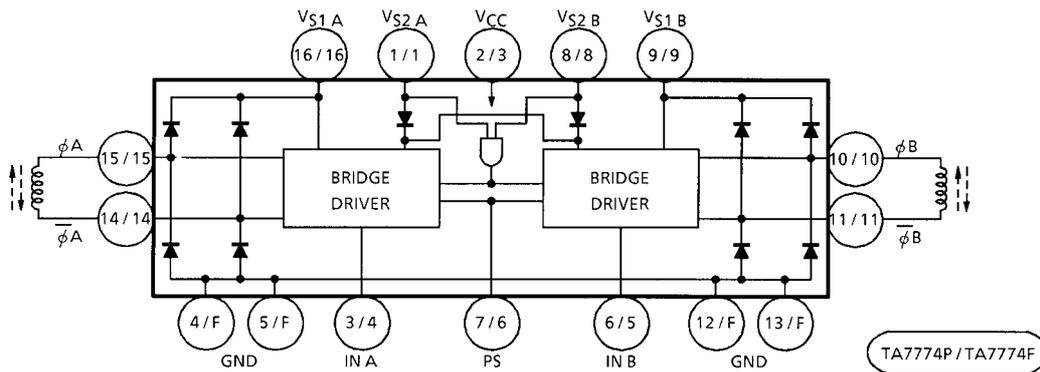
Note: Pin(2), (7), (12), (13) of TA7774F are all NC and Heat Fin is connected to GND.
