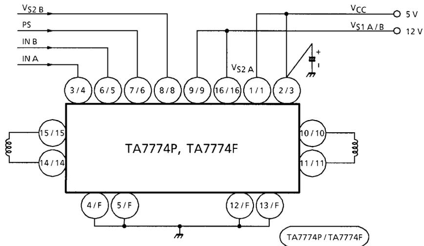
Note: Utmost care is necessary in the design of the output line,  $V_S$  and GND line since IC may be destroyed due to short-circuit between outputs, air contamination fault, or fault by improper grounding.
