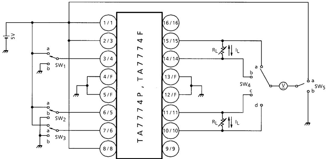
Note: Calibrate  $I_L$  to 20 / 100 mA by  $R_L$ .
