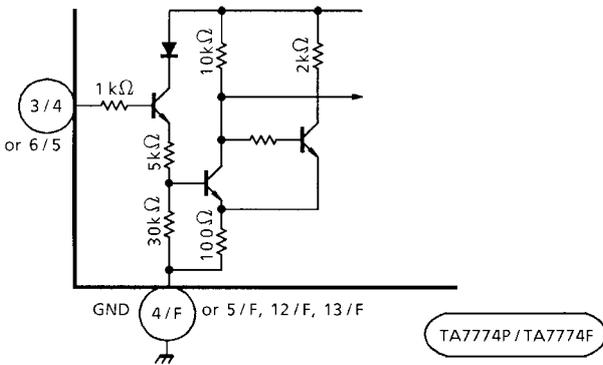
**INPUT CIRCUIT VS2 A or VS2 B**
