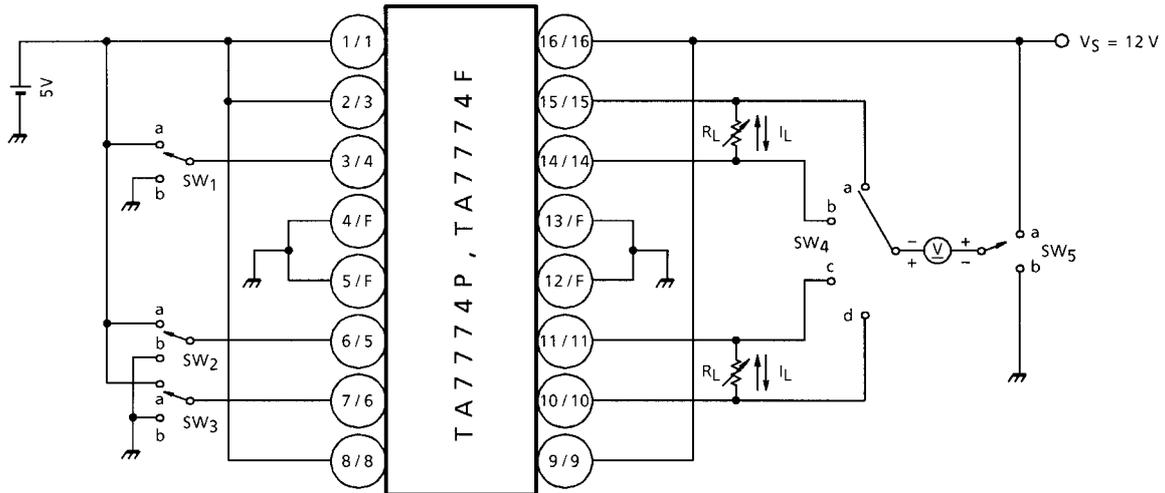
Note: Calibrate  $I_L$  to 0.4 / 0.1 A by  $R_L$ .
