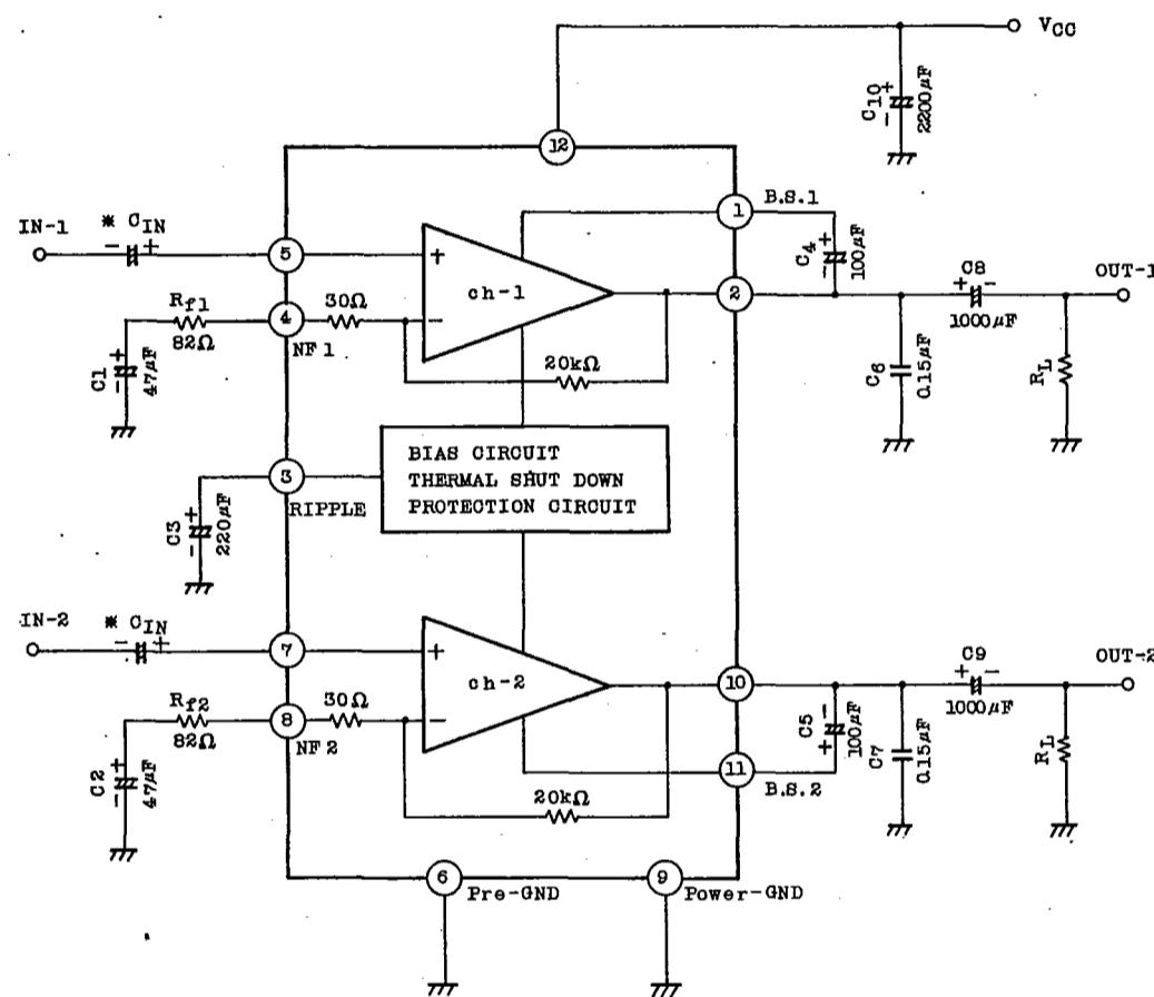
\* This IC can be used without coupling capacitor ( $C_{in}$ ). If volume slide noise occurred by input offset voltage is undesirable, it needs to use the capacitor ( $C_{in}$ ).
