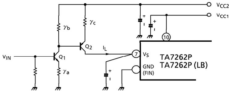
$$I_L \cong \frac{\gamma_b}{\gamma_a \gamma_c} \cdot V_{IN} - \frac{1}{\gamma_c} \left( \frac{\gamma_b}{\gamma_c} \cdot V_{BE1} + V_{BE2} \right)$$
