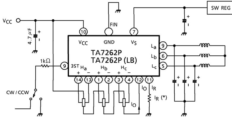
(\*) Hall sensor driving current ( $I_O$ ) can be changed by  $I_R$ . Refer to  $I_R$  vs  $I_O$  characteristics.
