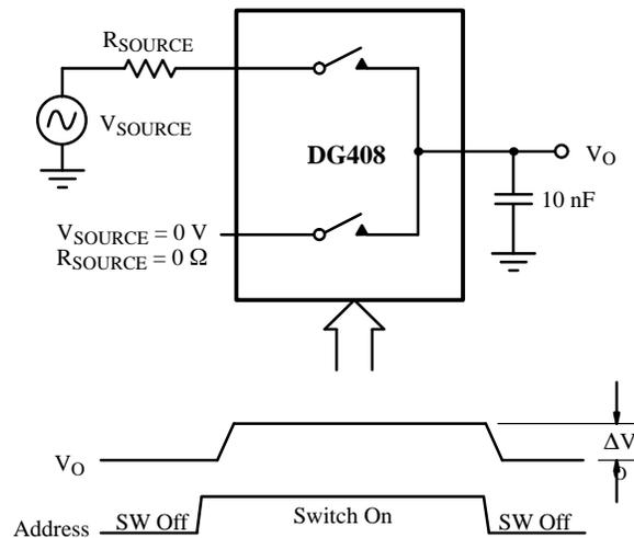
**Figure 7.** Charge Injection Test Circuit
