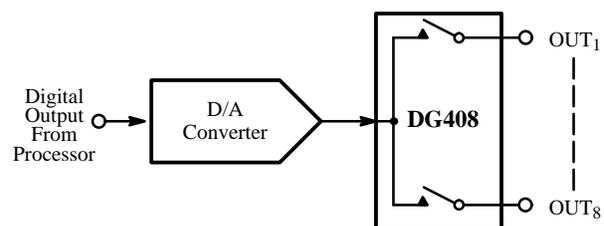
**Figure 9.** Using the DG408 as a Demultiplexer
