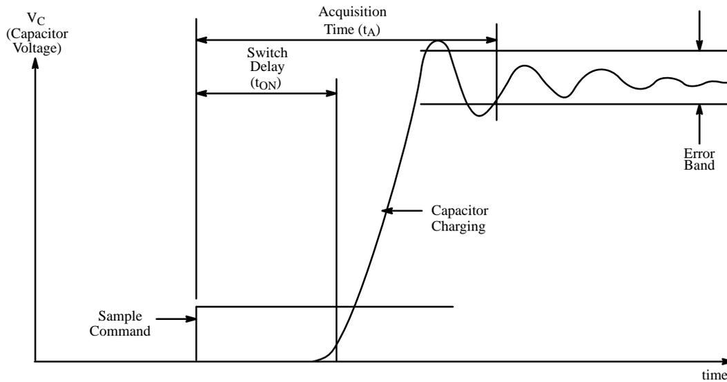
**Figure 11.** Acquisition Time of a Sample/Hold System
