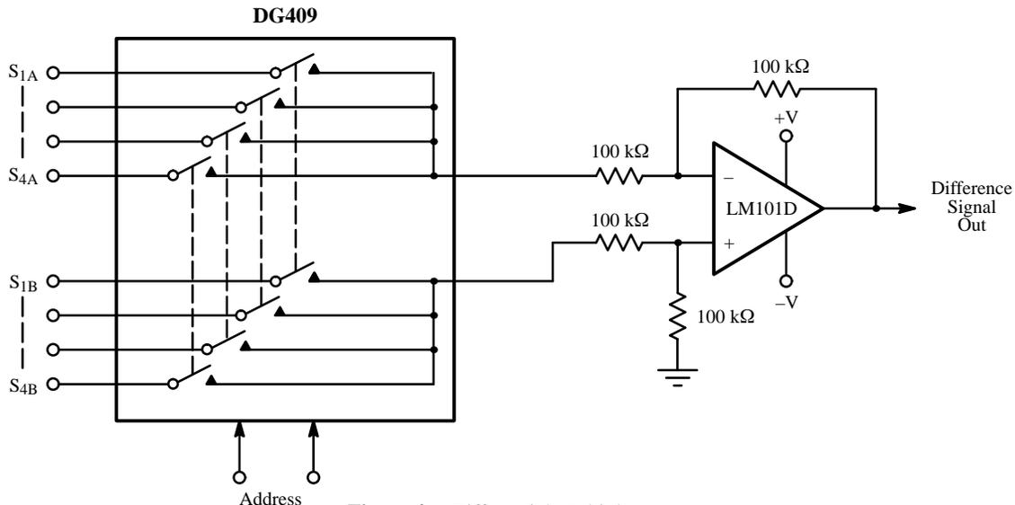
**Figure 4.** Differential Multiplexer
