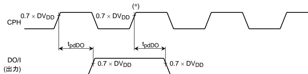
Note: Timing for loading OUT379 to OUT384
