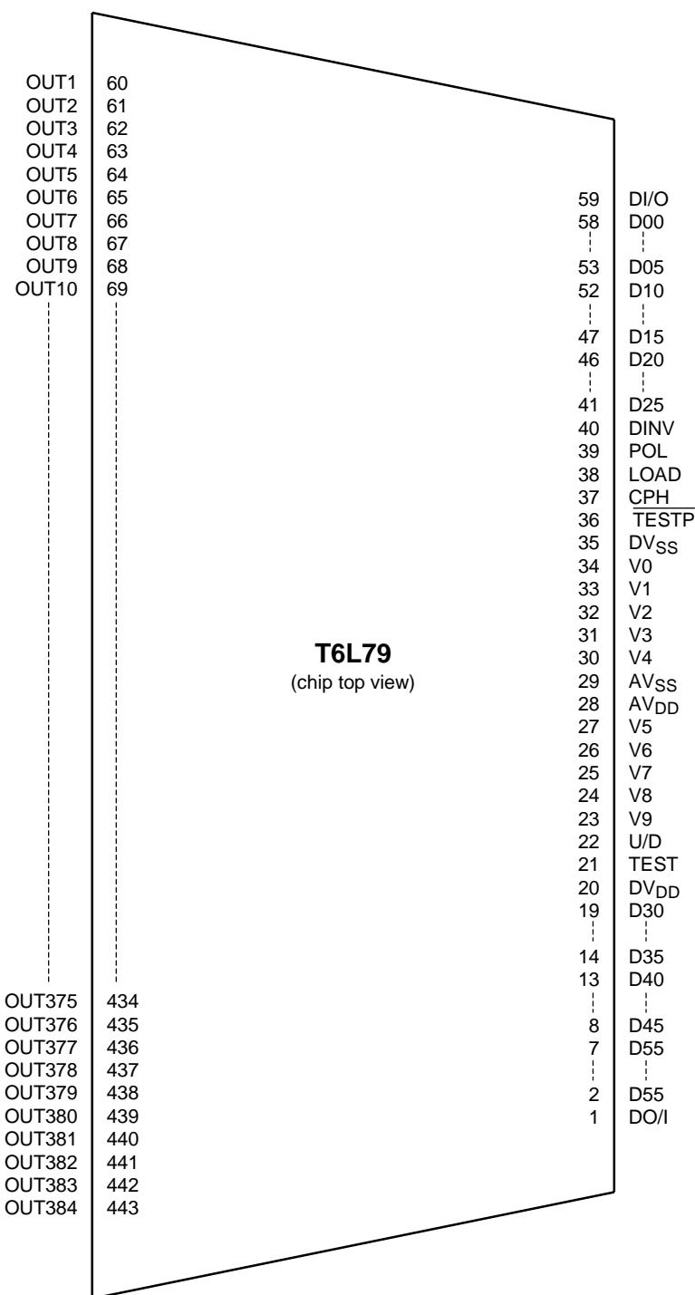
The figure above shows an example of the pin assignment in the TCP. It does not specify the pad layout on the chip. For the latest TCP specifications, contact Toshiba or your local sales office.
