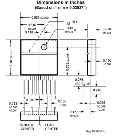
NOTE: Exact body and lead configuration at vendor's option within limits shown.
