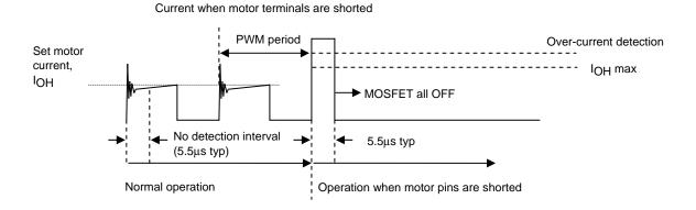
Overcurrent detection begins after an interval of no detection (a dead time of 5.5µs typ) during the initial ringing part during PWM operations. The no detection interval is a period of time where overcurrent is not detected even if the current exceeds IOH.
