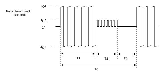
Figure 1 Motor Current Timing
