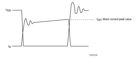
Figure 2 Output Current, I<sub>D</sub>, and Voltage, V<sub>DS</sub>, Waveforms 2 of the STK672-6\*\* Series when Driving a 2-Phase Stepping Motor with Constant Current Chopping
