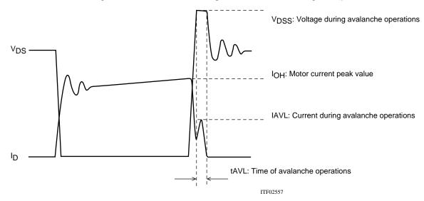
Figure 1 Output Current, ID, and Voltage, VDS, Waveforms 1 of the STK672-6\*\* Series when Driving a 2-Phase Stepping Motor with Constant Current Chopping
