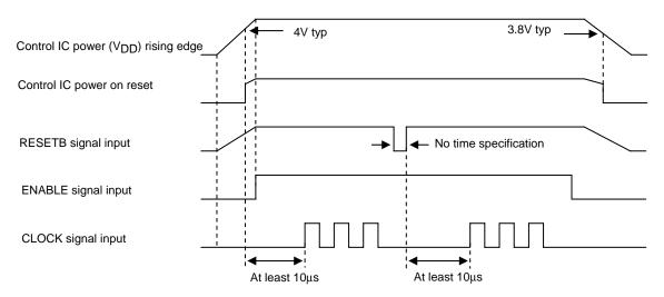
ENABLE, CLOCK, and RESETB Signals Input Timing
