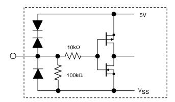
All input pins of this driver support schmitt input. Typ specifications at  $Tc = 25^{\circ}C$  are given below. Hysteresis voltage is 0.3V (VIHa-VILa).
