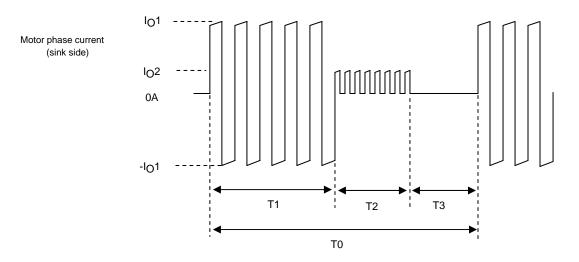
Figure 1 Motor Current Timing
