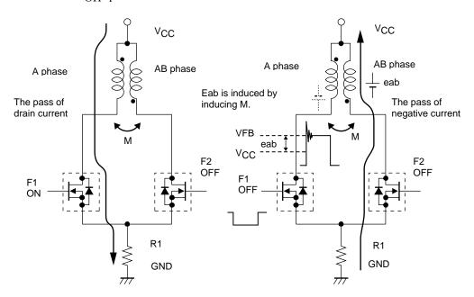
The oscillating voltage in excess of VFB is caused by LCRM (inductance, capacitor, resistor, mutual inductance) oscillation that includes micro capacitors C, not present in the circuit. Since M is affected by the motor characteristics, there is some difference in oscillating voltage according to the motor specifications. In addition, constant voltage drive without constant current drive enables motor rotation at  $V_{CC} \ge 0V$ .
