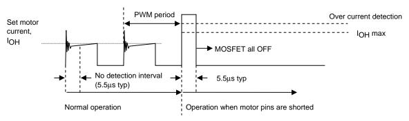
Over current detection begins after an interval of no detection (a dead time of  $5.5\mu s$  typ) during the initial ringing part during PWM operations. The no detection interval is a period of time where over current is not detected even if the current exceeds IOH.
