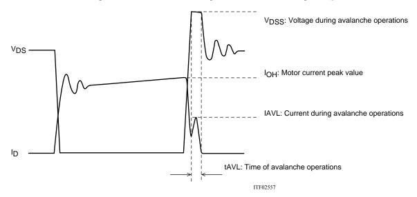
Figure 1 Output Current, I<sub>D</sub>, and Voltage, V<sub>DS</sub>, Waveforms 1 of the STK672-6\*\* Series when Driving a 2-Phase Stepping Motor with Constant Current Chopping
