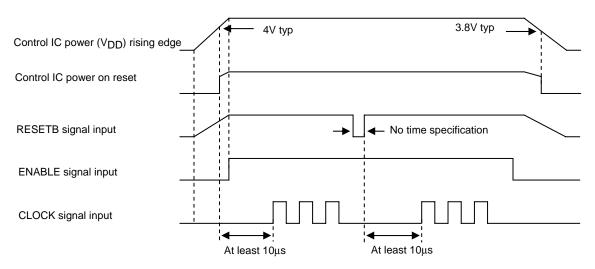
ENABLE, CLOCK, and RESETB Signals Input Timing
