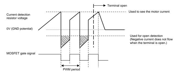
When the current level drops, the difference with the GND potential decreases, making detection difficult. The motor current that can be detected by motor terminal open detection is 0.25A or more with the STK672-612B-E.
