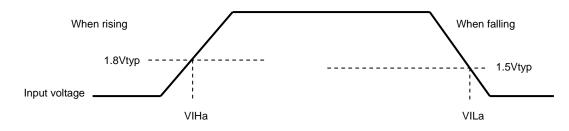
Input voltage specifications are as follows.  $V_{IH}$ =2.5Vmin
