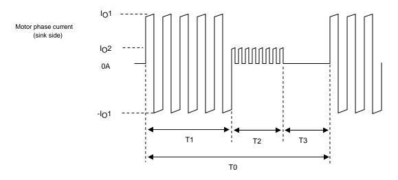
Figure 1 Motor Current Timing
