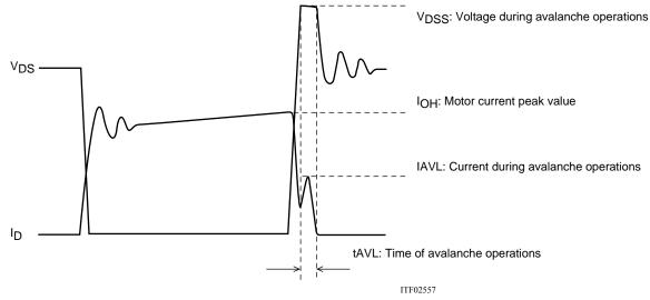
Figure 1 Output Current, I<sub>D</sub>, and Voltage, V<sub>DS</sub>, Waveforms 1 of the STK672-4\*\* Series when Driving a 2-Phase Stepping Motor with Constant Current Chopping
