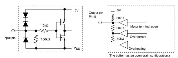
The input pins of this driver all use Schmitt input. Typical specifications at Tc=25°C are given below. Hysteresis voltage is 0.3V (VIHa-VILa).
