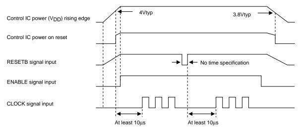
ENABLE, CLOCK, and RESETB Signals Input Timing
