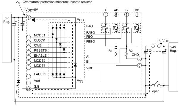
Overcurrent protection measure: Insert a diode.
