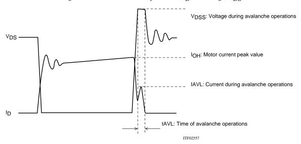
Figure 1 Output Current, I<sub>D</sub>, and Voltage, V<sub>DS</sub>, Waveforms 1 of the STK672-2\*\* Series when Driving a 2-Phase Stepping Motor with Constant Current Chopping
