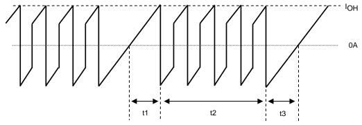
Figure 1 Motor COM current waveform model
