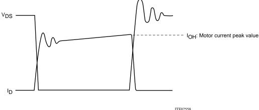
Figure 2 Output Current, I<sub>D</sub>, and Voltage, V<sub>DS</sub>, Waveforms 2 of the STK672-2\*\* Series when Driving a 2-Phase Stepping Motor with Constant Current Chopping
