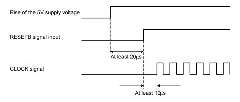
Figure 2 RESETB and CLOCK Signals Input Timing
