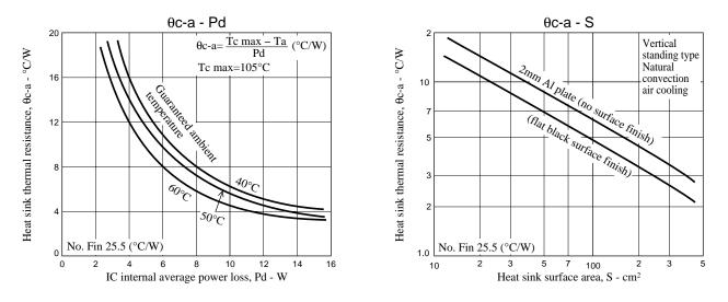
Next we determine the usage conditions with no heat sink by determining the allowable hybrid IC internal average loss from the thermal resistance of the hybrid IC substrate, namely 25.5°C/W.
