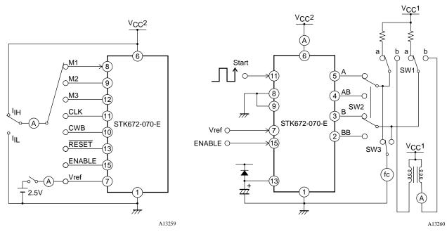
For Ioave measurement: Set switch SW1 to the b position, provide the Vref input and switch over switch SW2. For fc measurement: Set SW1 to the a position, set Vref to 0V, and switch over switch SW3. For I<sub>CC</sub> measurement: Set the ENABLE input to the low level.
