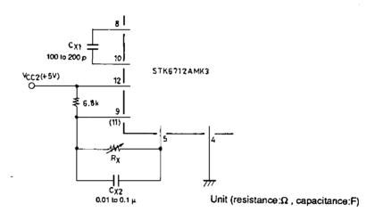
Fig. 10 Motor Hold Noise Countermeasure
