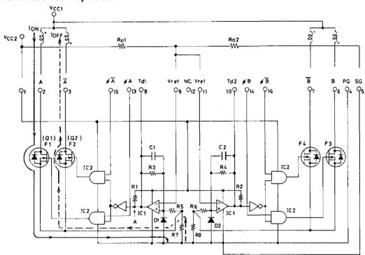
Fig. 1 STK6712AMK3 Internal Equivalent Circuit
