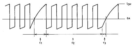
Fig. 7 Motor Output Current Waveform (model)
