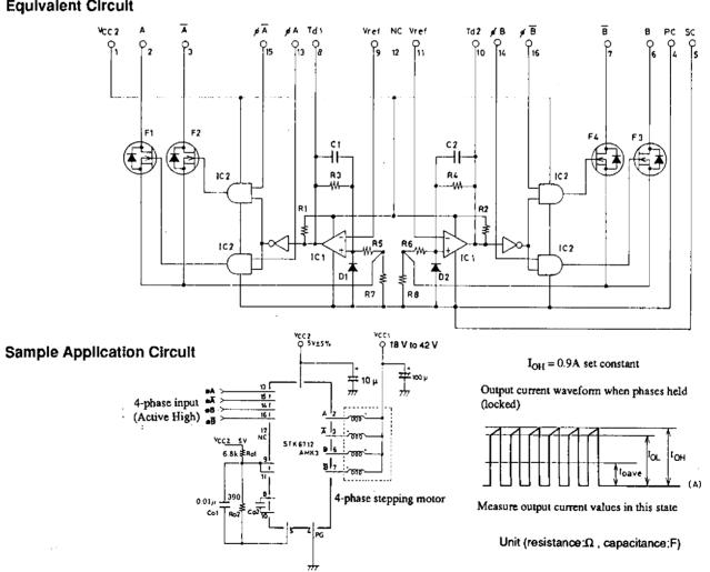
Note ~ For reference, when  $I_{OH}~$  1.0 A,  $R_{O1}$  = 6.8  $k\Omega$  and  $R_{O2}$  = 390  $\Omega.$
