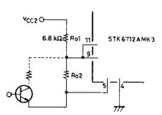
Fig. 4 Vref Peripheral Circuit
