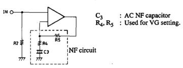
• VG settings are obtained using  $R_4$  and  $R_5$  according to the following equation:
