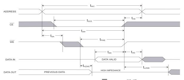
Figure 11. SRAM Write Cycle 2: CE Controlled [15, 16]
