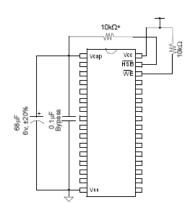
In system power mode, both V $_{CC}$  and V $_{CAP}$  are connected to the +5 V power supply without the 68  $\mu$ F capacitor. In this mode, the AutoStore function of the STK14C88-5 operates on the stored system charge as power goes down. The user must, however, guarantee that V $_{CC}$  does not drop below 3.6 V during the 10 ms STORE cycle.
