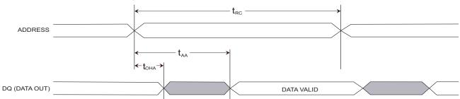
Figure 9. SRAM Read Cycle 2:  $\overline{\text{CE}}$  and  $\overline{\text{OE}}$  Controlled [9]
