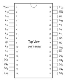
Figure 1. Pin Diagram: 32-Pin LCC
