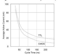
Figure 6. Current Versus Cycle Time (WRITE)
