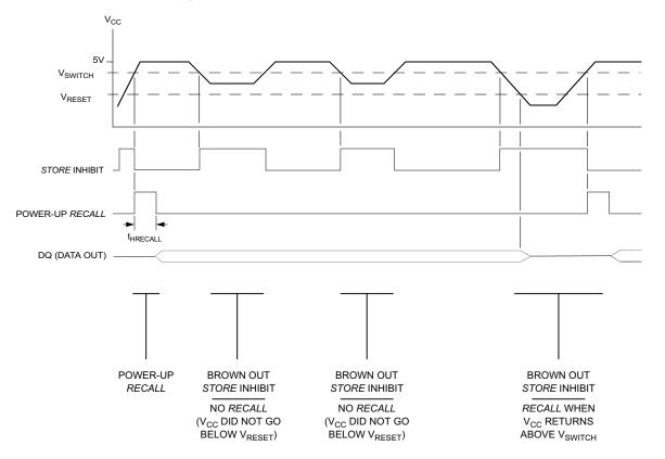
Figure 10. AutoStore INHIBIT/Power Up RECALL
