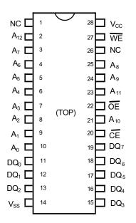
Figure 2. Pin Diagram - 28-Pin LLC
