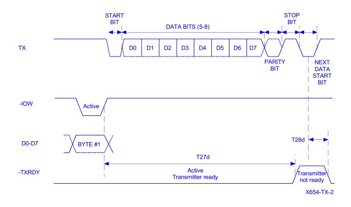
Transmit ready timing in none FIFO mode
