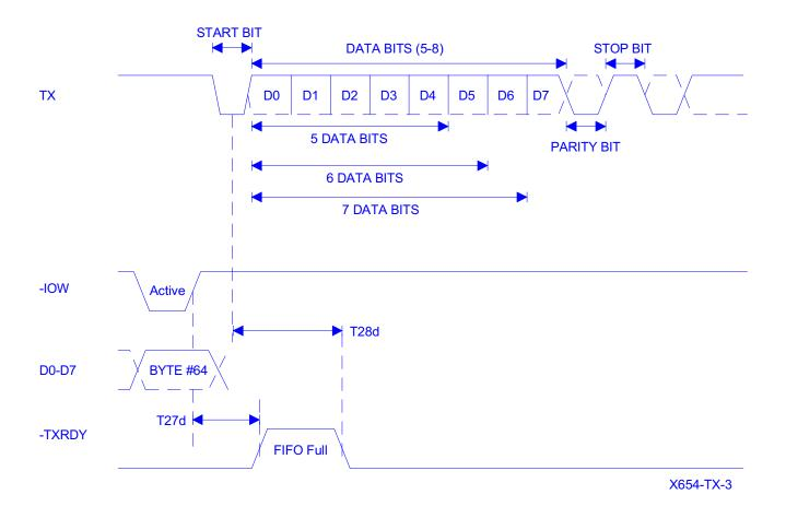
Transmit ready timing in FIFO mode
