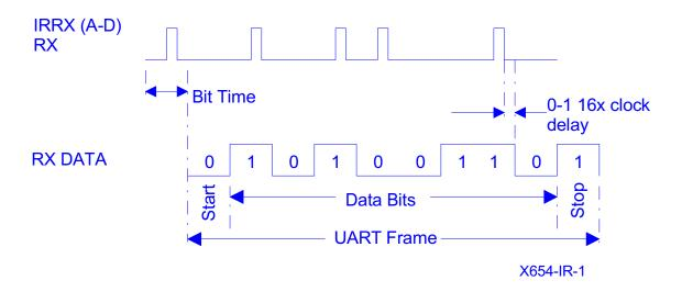
Infrared receive timing
