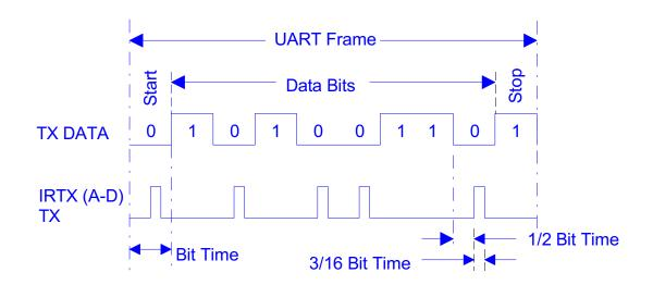
Infrared transmit timing
