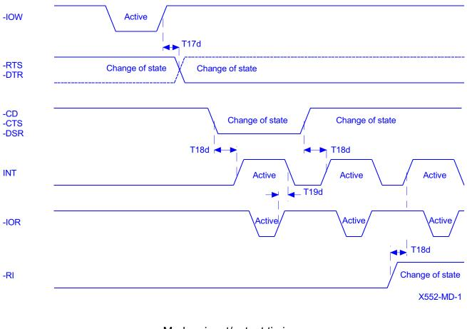
Modem input/output timing
