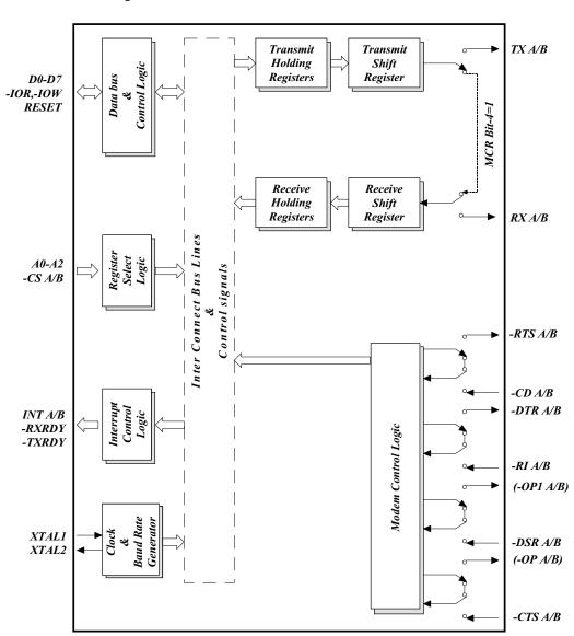
Figure 4, INTERNAL LOOP-BACK MODE DIAGRAM
