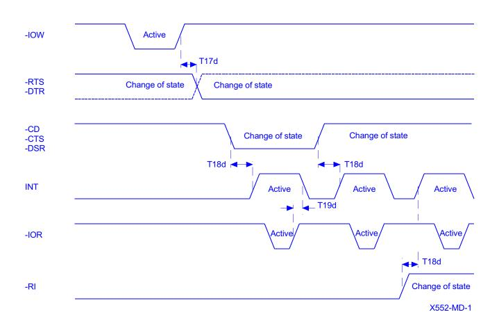
Modem input/output timing
