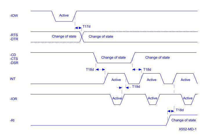
Modem input/output timing
