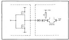
Fig. 3 CMOS and TTL compatible control input
