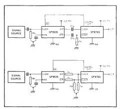
Fig. 6 Methods of preventing self-oscillation
