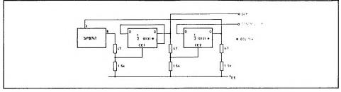
Fig. 6 Divide-by-12/14. Control loop delay time approximately 40ns.
