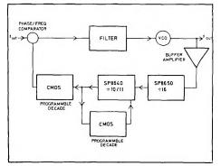
Fig. 5 A low power synthesiser loop
