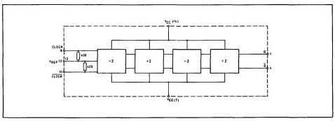
Fig. 2 Functional diagram
