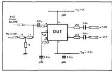
Fig. 3 Toggle frequency test circuit
