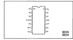
Fig. 1 Pin connections
