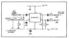
Fig. 3 Toggle frequency test circuit
