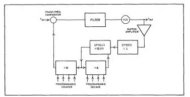
Fig. 6 A 1.5GHz synthesiser loop
