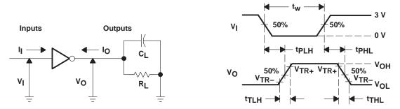
NOTES: A. The pulse generator has the following characteristics: For C<sub>L</sub> < 1000 pF: t<sub>W</sub> = 4  $\mu$ s, PRR = 250 kbit/s, Z<sub>O</sub> = 50  $\Omega$ , t<sub>r</sub> = t<sub>f</sub> < 50 ns. For C<sub>L</sub> = 2500 pF: t<sub>W</sub> = 8  $\mu$ s, PRR = 125 kbit/s, Z<sub>O</sub> = 50  $\Omega$ , t<sub>r</sub> = t<sub>f</sub> < 50 ns. B. C<sub>L</sub> includes probe and jig capacitance.
