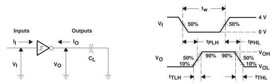
NOTES: A. The pulse generator has the following characteristics:  $t_W = 4 \mu s$ , PRR = 250 kbit/s,  $Z_O = 50 \Omega$ ,  $t_r = t_f < 50 ns$ . B. CL includes probe and jig capacitance.
