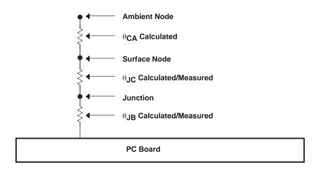
Figure 12. Thermal Resistance
