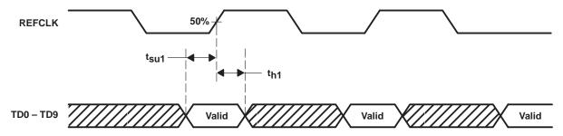
Figure 4. Transmit 10-Bit Interface Timing Waveforms
