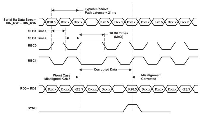
Figure 2. Word Realignment Timing Characteristics Waveforms
