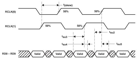
Figure 6. Receiver Interface Timing Waveforms
