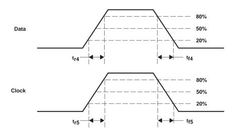
Figure 5. Receiver Data Measurement Levels
