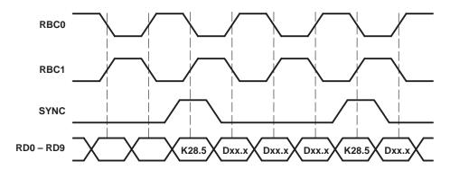
Figure 1. Synchronous Timing Characteristics Waveforms
