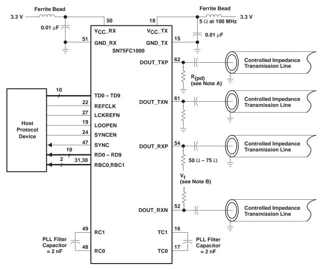
NOTES: A. R(pd) – This value is set to match the falling edge to rising edge transistion times, typically 150  $\Omega$ .
