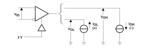
Figure 1. V<sub>OH</sub> and V<sub>OL</sub> Test Circuit
