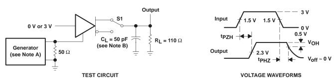
NOTES: A. The input pulse is supplied by a generator having the following characteristics: PRR  $\leq$  1 MHz, 50% duty cycle, t<sub>r</sub>  $\leq$  6 ns, t<sub>f</sub>  $\leq$  6 ns, Z<sub>O</sub> = 50  $\Omega$ .
