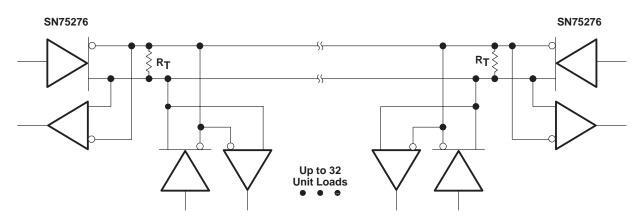
NOTE A: The line should be terminated at both ends in its characteristic impedance. Stub lengths off the main line should be kept as short as possible ( $R_T = Z_O$ ).
