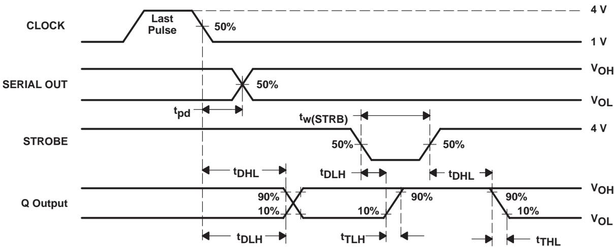
Figure 2. Switching Characteristics
