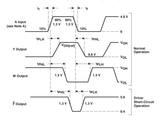
NOTE A: The input pulse is supplied by a generator having the following characteristics: PRR = 1 MHz, duty cycle = 50%,  $t_f \le 6$  ns,  $t_f \le$
