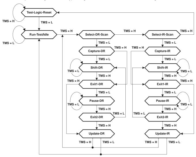
Figure 1. TAP-Controller State Diagram
