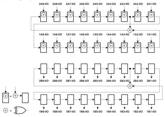
Figure 9. 18-Bit PSA/PRPG Configuration (1OEAB = 2OEAB = 0, 1OEBA = 2OEBA = 1)
