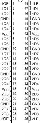
A buffered output-enable  $(\overline{OE})$  input can be used to place the eight outputs in either a normal logic state (high or low logic levels) or a high-impedance state. In the high-impedance state, the outputs neither load nor drive the bus lines significantly. The high-impedance state and the increased drive provide the capability to drive bus lines without need for interface or pullup components.
