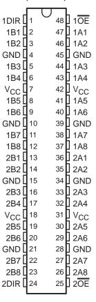
Active bus-hold circuitry is provided to hold unused or floating data inputs at a valid logic level.
